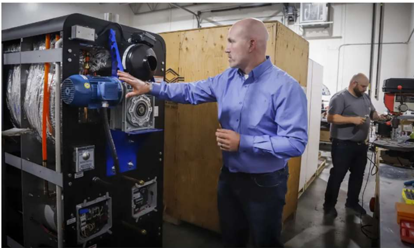
Jaeson Cardiff, left, CEO of CleanO2, explains his CARBiN-X technology that uses a chemical process to convert CO 2 captured from heating system exhaust into a stable carbonate used in soaps and detergents, at the company's facility in Calgary, Alta., Thursday, July 22, 2021.
